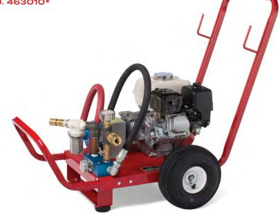
A durable, value-driven pump that is easy to maintain and can test pressure up to 300 PSI. Capable of pumping up to 5.4 gallons per minute, this pump features an inline strainer with stainless steel mesh filter and clear bowl.
