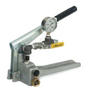
Manual test pump that is ideal for testing residential water lines, small pressure tanks, sprinkler and boiler systems. The durable, handheld unit can test lines up to 300 PSI and features a 3/4" garden hose female inlet and 9/16"-18 JICF male outlet. A 10-foot output hose is also included.
