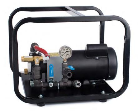
A smooth operating twin piston pump capable of testing line from O to 500 PSI while pumping 3 gallons of water per minute.
