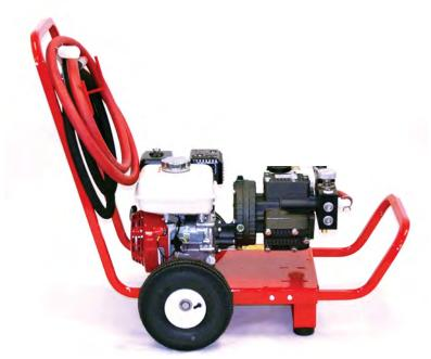
Features a triple diaphragm pump that can handle up to 10 percent chlorine solution. This rugged, durable pump can run dry and is capable of handling the toughest jobs. The pump can be preset to test lines from 0 to 500 PSI while pumping up to 10 gallons per minute.
