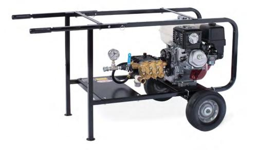
A triplex piston pump capable of testing lines from 150 to 3,000 PSI while pumping 3.5 gallons of fluid per minute. Designed for a smoother operation, the 373080 is ideal for industrial use.
